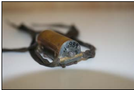
Figure 4. Transmitter removed from the Faata male; just some down where the antenna should be.
